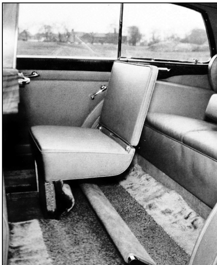
The original Silky Crushed Mohair and Mouton bordered overlay as used in the rear compartment of our Rolls-Royce Silver Wraith H.J. Mulliner Limousine. The remainder of the trim in this commercial livery model is tan Connolly leather seats and West of England cloth on the headlining and sidewalls..
