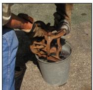
Another application, for which I have found this approach useful, is with nut removal from a bolt. A similar approach, without water, works for removing broken stud bolts on an item such as an engine head. In this case, you place a nut directly over the stud bolt that is probably broken off flush with the head. You then arc weld the nut to the stud bolt, completely filling the inside of the nut with weld. Let the area cool naturally and the stud bolt will turn right out with a wrench.
