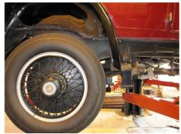
Rolls Royce Phantom I positioned on car lift to allow negative weight on leaf springs.
